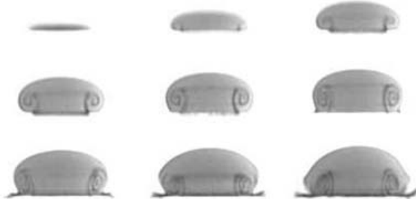
FIGURE 4. Series of images taken at 24 frames per second from a typical experiment with a weak fountain. The source conditions were Fr_0 = 1.3 and Re_0 = 254 .
